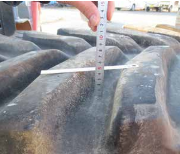
Fig. 1. How to measure the tread depth
