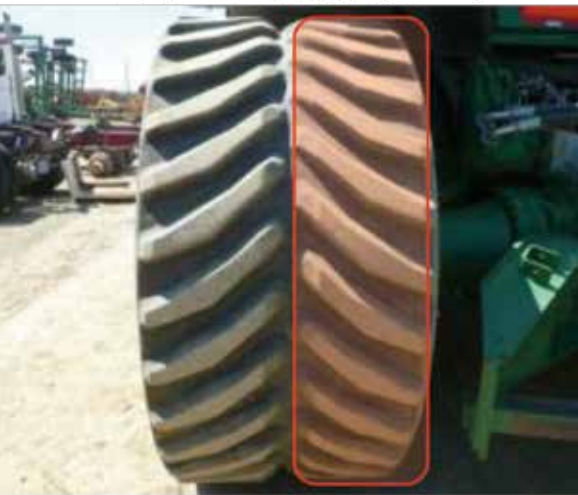
Fig. 1. Accelerated machine side tread wear
