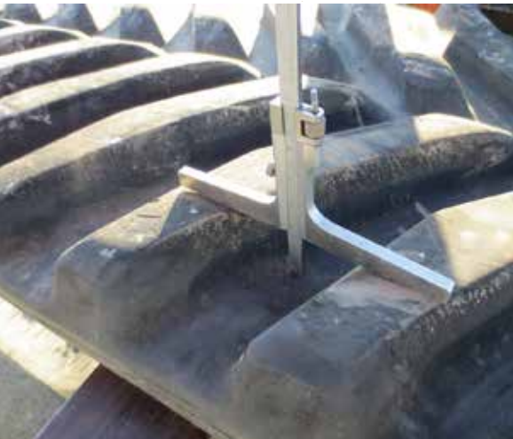
Fig. 1. How to measure the tread depth
