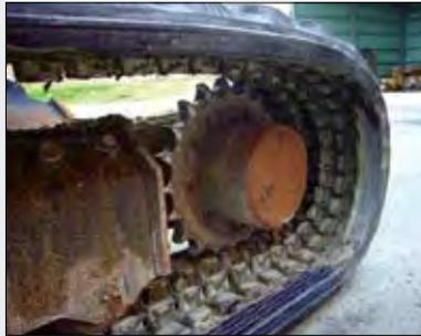
De-tracking at sprocket
