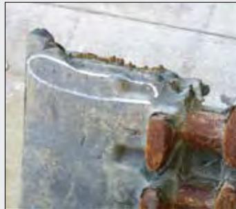
Steel cord breakage at end of overlap
